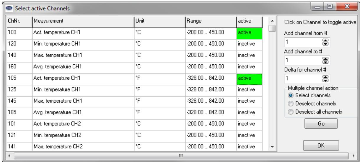
Here you are able to select the channels for query, either through clicking the corresponding channel in the list, or by using the “Multiple channel action” function with the channel numbers.
