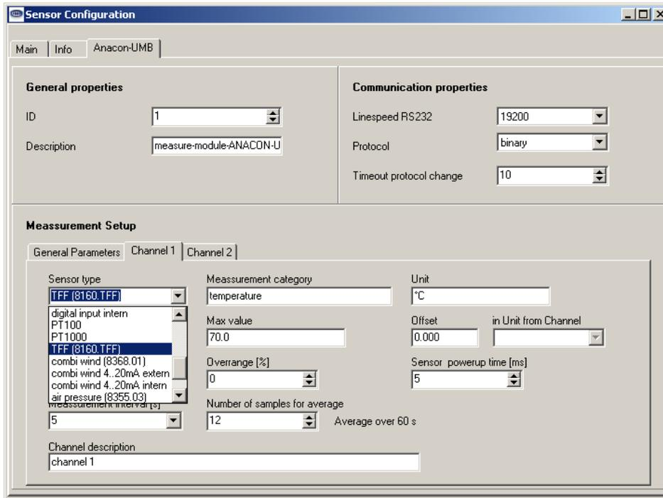
If necessary, set the ID, measurement interval and number of measurements for the min-, max- and average values:
