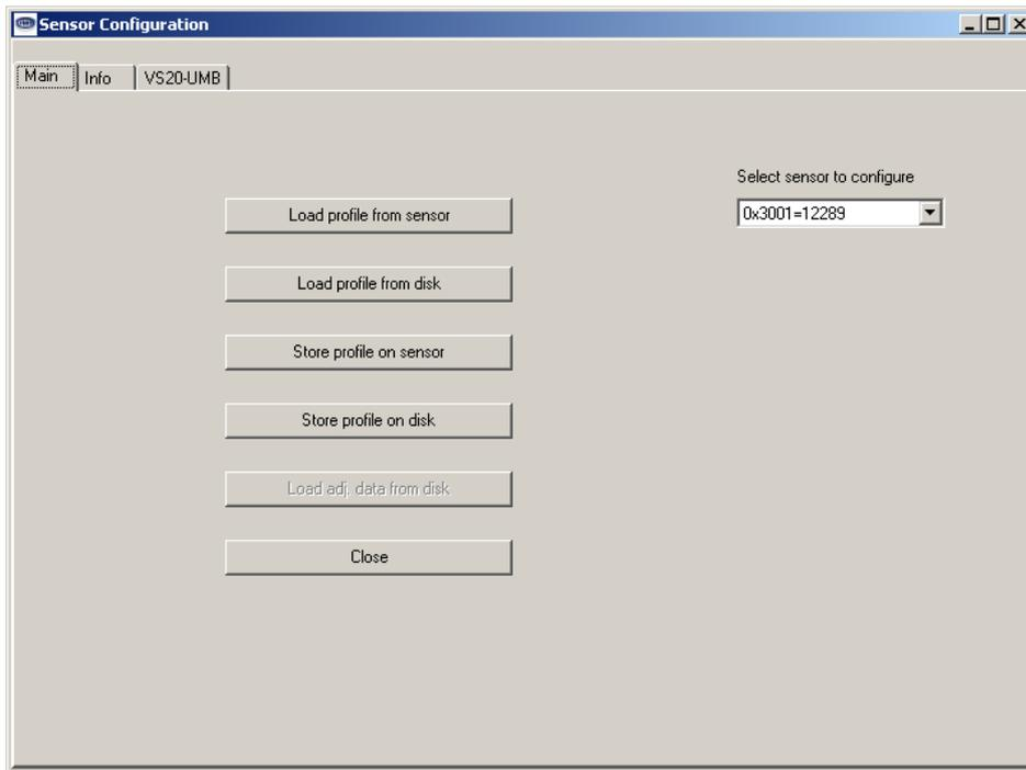
With ‚Store profile on disk‘ a sensor configuration might be stored on a hard drive. Stored configurations of sensors might be loaded with ‚Load profile from disk‘.
