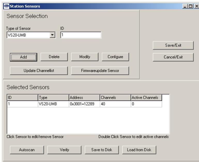
Choose 'Type of Sensor'; enter an ID and add it with 'Add' to the list. With 'Delete' sensors can be deleted, with 'Modify' a sensor in the list can be modified. The sensor shown in 'Sensor Selection' will be deleted or modified.
