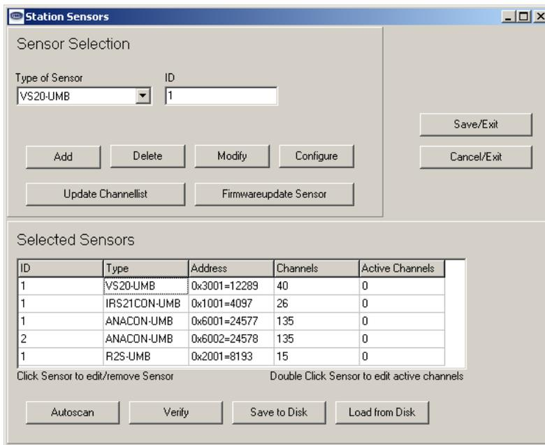
Select the appropriate sensor from the sensor list; the selected sensor is displayed in the 'Selected Sensors' section (VS20-UMB in the example).
