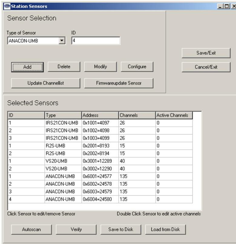
**ATTENTION:** When configuring new equipment please note that **new devices always have the ID 1!** If there are several sensors of the same type in a network it makes sense to configure the sensors individually with their corresponding ID's **before** commissioning the network.
