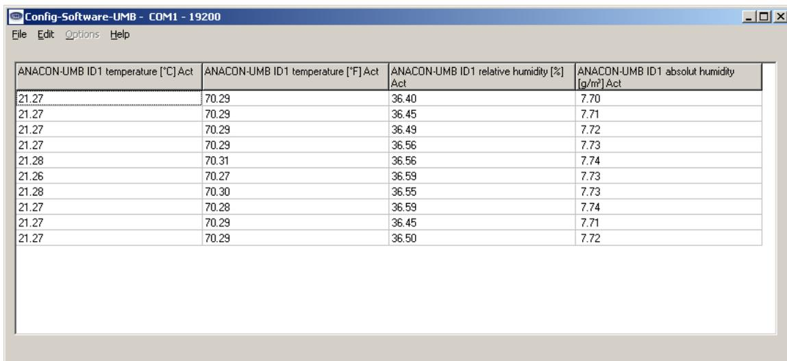
To change the sampling rate of the software click ,Edit' → ,Sampling Rate'. A sample rate of 1s does not correspond to the UMB-protocol. In the case of missing answers of the sensor it can lead to erroneous presentation of the received values.
