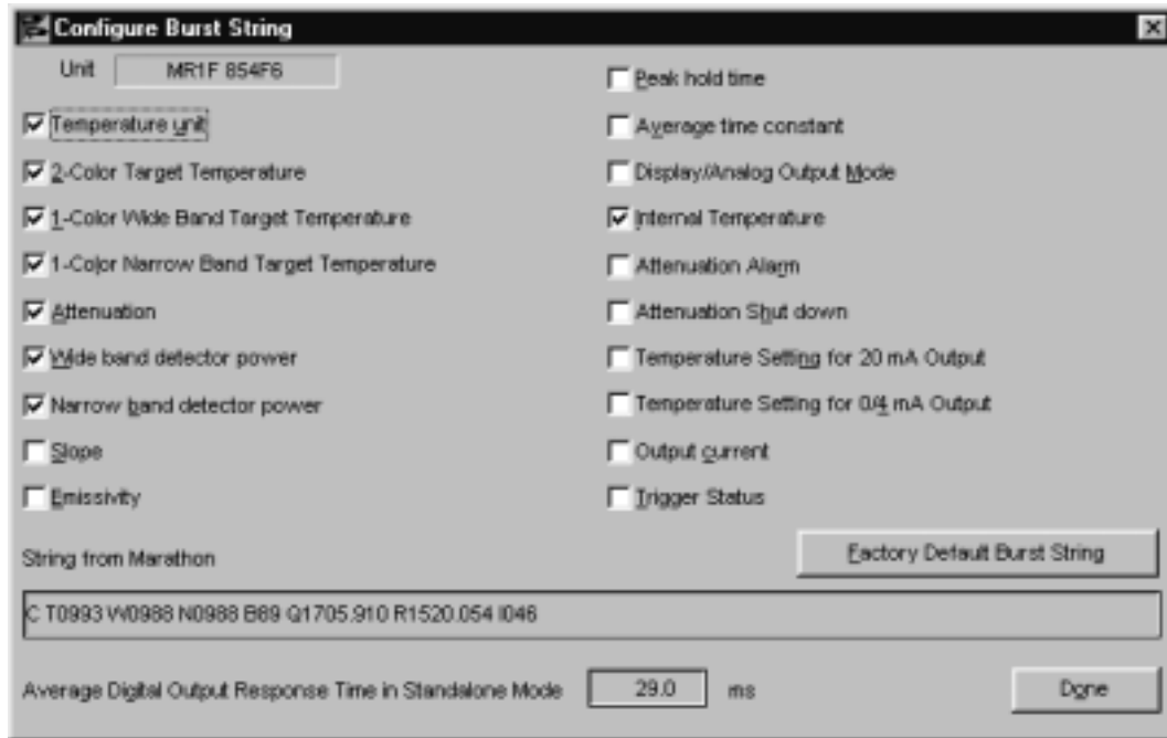
Figure 4-6: Configure Burst String Window
