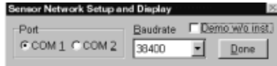
Figure 4-8: Sensor Network Communication Setup
