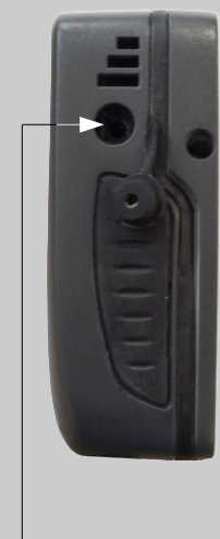
Jack connector (3.5) Input for Kistock-PC software
