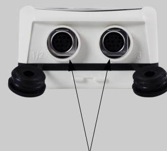
Mini-Din connectors for Pt100 probes
